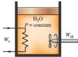
**Q-5** An insulated piston-cylinder device initially contains 1.8 kg of saturated liquid water at 120 °C. Now an electric resistor placed in the tank is turned on for 10 min until the tank contains saturated vapor and the volume quadruples. Determine a) the volume of the tank, b) the final temperature and c) the electrical power rating of the resistor.
