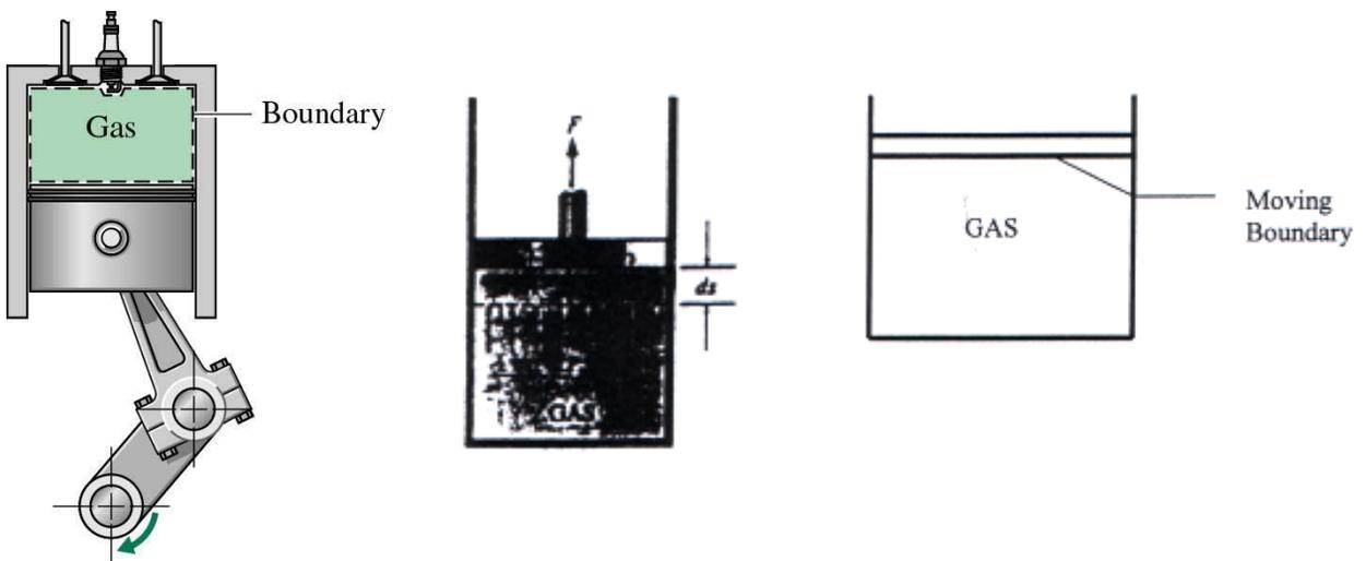
If piston is allowed to move a distance  $ds$  in a quasi-equilibrium manner, the differential work done during this process is
