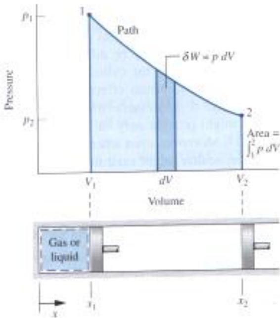
Expansion work done by the gas on the piston from state 1 to 2 can be calculated as
