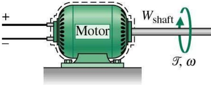
Shaft work (Power transmitted by a shaft).
