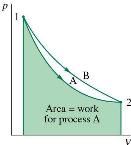
In general as piston moves from state **1 to 2**, relation between pressure and volume could be different. That means **P-V curve** may follow different paths from state **1** and **2**. Hence, even though processes take place between the same states, area under the curves will be different. This yields different values for the work. This result reveals that
