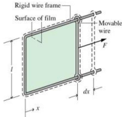
Stretching of a liquid film
