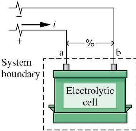
► When a **battery is charged electrically**, energy is transferred to the battery contents by work.
