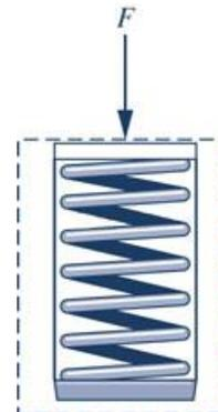
When a **spring is compressed**, energy is transferred to the spring by work
