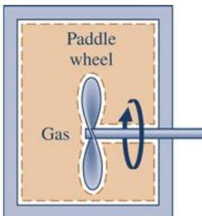
When a **gas in a closed vessel is stirred**, energy is transferred to the gas by work.
